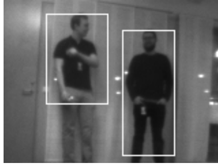
Figure 18: 160 \times 120 image captured by the camera on the AI-deck, showing two people where both are detected and identified as human bodies. The legs of the person to the left are cropped out by the detection algorithm whereas the bounding box surrounding the person to the right captures the full body.
