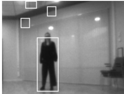
Figure 19: Example when the detection model successfully detects a human present in the image, but also missclassifies parts of the background to be human bodies.
